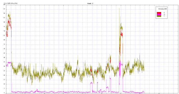
Figure 13. Curves P , Q and S recorded by MIS-2S being installed on 0.4 kV pole - channel 2
