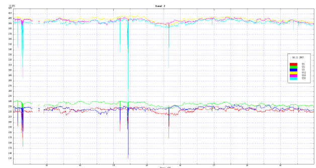
Figure 4. Phase and line voltages recorded on a pole of LV feeder of TS 10/0.4 kV "V. Jovanovic" - 06.11.2007.
