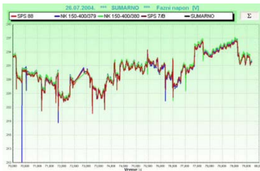
Fig. 3 Diagram of Voltage Changes on Induction Motor Connectors
